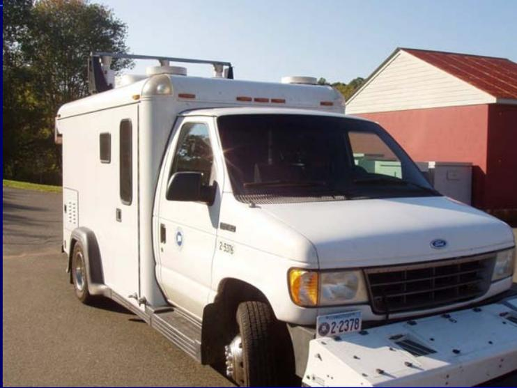
This is a typical photolog van. It's equipped with cameras, a gyroscope, sensors, and computer hardware and software to collect all the data previously mentioned. This is one of ours and it is called an Automatic Road Analyzer or ARAN for short.
